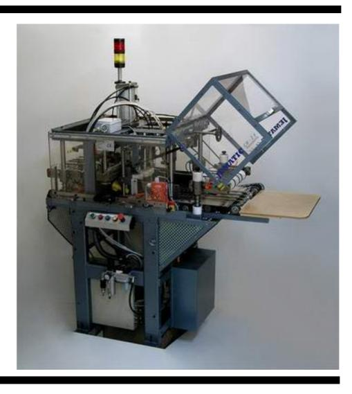
Floor stand model with staple hold and hardened knife for long and trouble free work.
